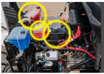
Power Electronics/Motor Coolant Reservoir (Top Left) Cab Heat Reservoir (Middle) Battery Chiller Reservoir (Bottom Right)
